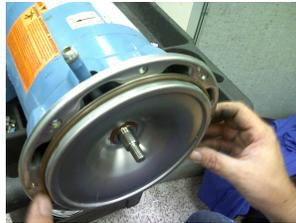
10. Check both seating surfaces to assure they are free of any foreign matter, grease, and finger prints. Slide the mechanical seal rotary assembly on the shaft. Ensure that there is no lubricant on the seating surfaces between the mechanical seal rotary assembly and the stationary seat.
