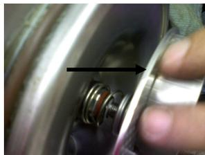
12. Lubricate and install a new casing O-ring to the Seal Housing.
