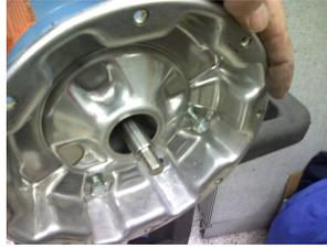
9. Install the seal housing with the new mechanical seal stationary seat into the motor adaptor. Lubricating the shaft with some viton lubricant can aid in sliding the assembly into place. Seating surfaces should not be lubricated.
