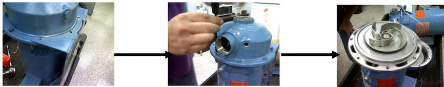
3. Remove the Impeller from the shaft. To do this you will need to remove the end cap from the cooling fan. To keep the impeller shaft from rotating, you can apply a 1/2" wrench to the end of the shaft at the cooling fan to apply counterforce and keep the shaft from turning. Use a straight bar like a long screwdriver to break the impeller free. From that point, you should be able to turn the impeller by hand. In some cases, you may need to heat the impeller/shaft to loosen the loctite.
