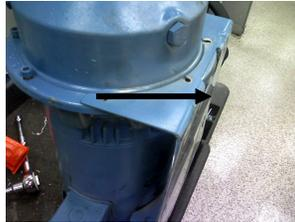
14. Reinstall the motor cooling fan guard.
