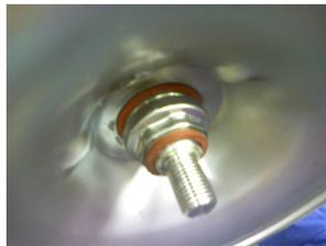
11. Install the washer on the end of the shaft that was previously removed during the disassembly procedure. Install the spring. Make sure that the spring engages the shoulder of the seal head. When installing the impeller, ensure the threads are clean and apply a small amount of Loctite 7649 primer to the threads. Wait about 2-3 minutes and use either Loctite 242 or 243 on the threads, screw the impeller in place. Torque the impeller to a value of 144 in-lbs.
